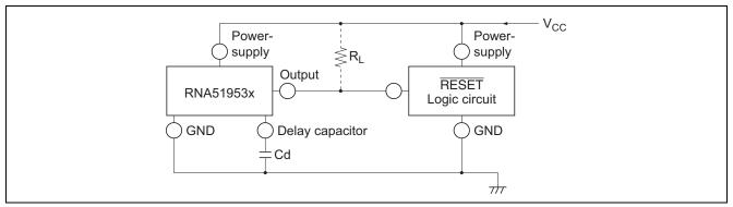
Figure 1 Reset Circuit of RNA51953
