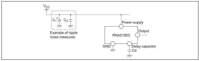
Figure 3 Example of Ripple Noise Measures
