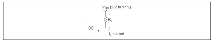
Figure 6 Output Load Resistance R<sub>L</sub>
