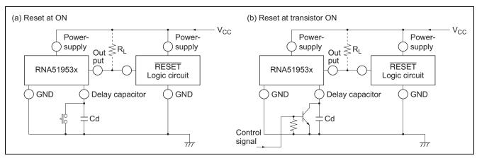
Figure 2 Case of Using Reset Signal except Supply Voltage in the RNA51953
